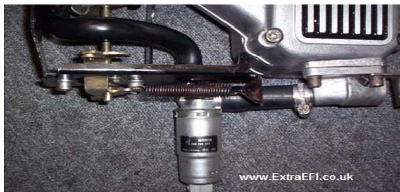
The original pipe on a Rover/TVR V8 setup that fed the stepper has been cut to allow the bosch idle valve to fit in line. The stepper motor can be left in place.
